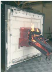
These pictures show the firestopping quality of the Actifoam® rubber. Even with the firestop placed at the exposed side, a two hour fire exposure is possible.
